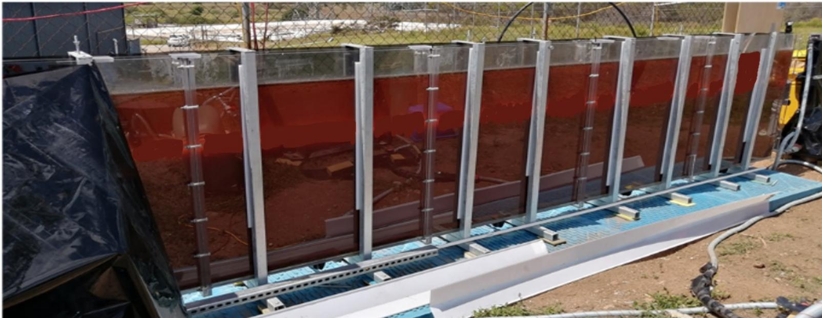
$V = 950 \text{ L}; \text{HRT} = 1.0\text{-}5.7 \text{ d}; \text{OLR} = 0.8\text{-}2.2 \text{ g COD}\cdot\text{L}^{-1}\cdot\text{d}^{-1}$
